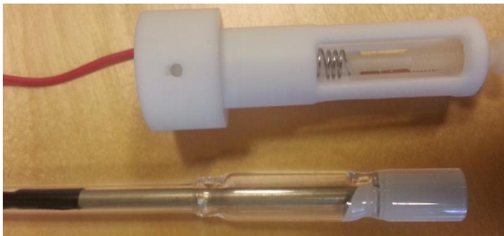
Figure 1. Homebuilt holder used in the electrografting of German silver.
