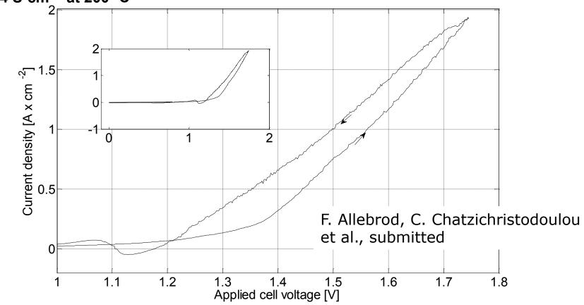
Cyclic voltage sweep on a cell with nickel-based gas diffusion electrodes. Current densities of 1.0 A·cm<sup>-2</sup> at 1.5V and 1.9 A·cm<sup>-2</sup> at 1.75V. 3.7 MPa and 241 °C. Calculated EMF 1.2 V. 1 cm<sup>2</sup> button cell.
